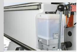
Lubrication is accomplished over central lubrication bars. This supports the high precision of movement and ensures long component service life. Manual or automatic central lubrication (both optional) also minimises maintenance (Fig. shows manual central lubrication).
